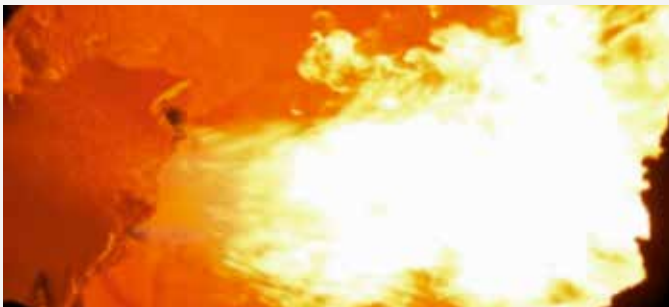
The picture shows the burner flame at the start of the experiment at 175 l/h, without EuroAd.
